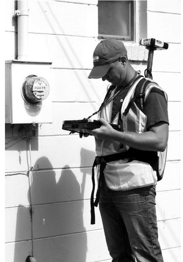
A Davey Resource Group employee is shown taking a GPS reading at a member's meter for the co-op's GPS mapping project. DRG was hired by the co-op to record the GPS coordinates of the utility's entire distribution system.
