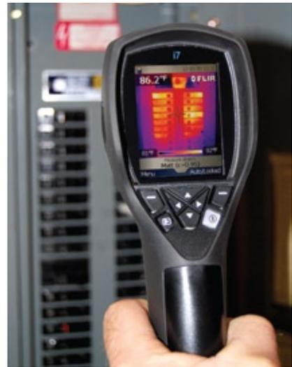
A thermal imaging camera is shown taking a reading of a breaker panel.
